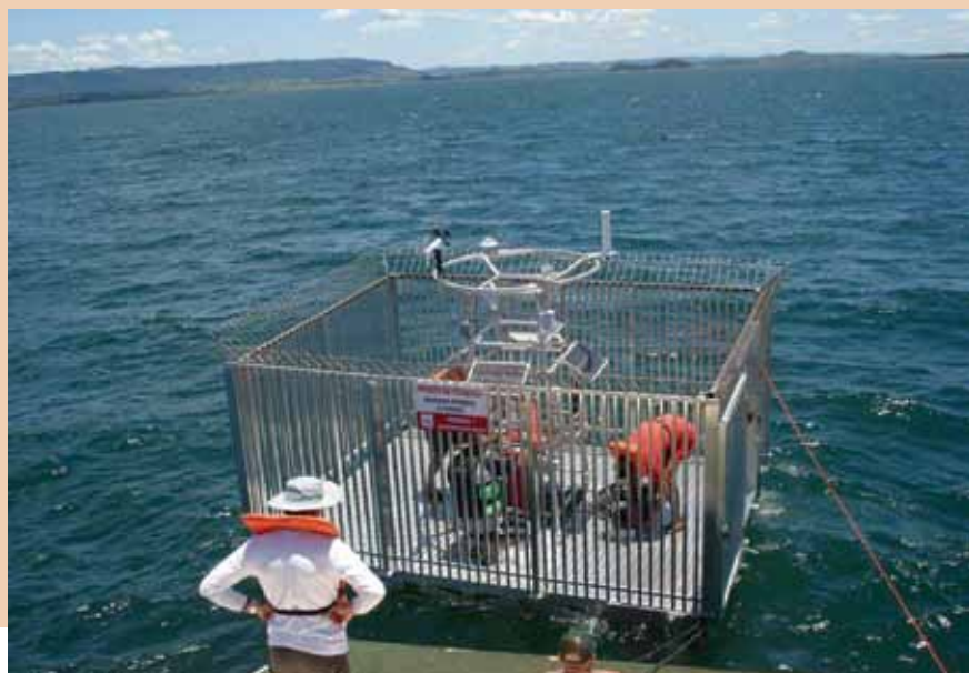
Telemetric Monitoring System (SIMA) deployed at the Itumbiara Reservoir, Goiás, Central Brazil.
