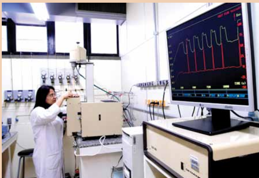
Thermogravimetric analysis of an oxygen carrier in the combustion reaction.
