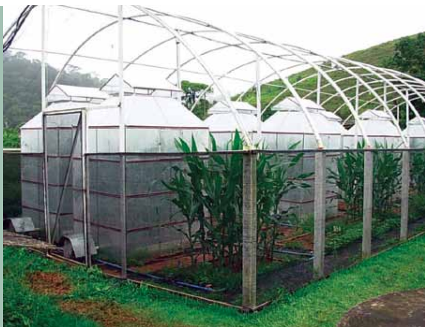
Open-top chambers used to simulate an atmosphere enriched by distinct levels of CO 2 resembling the IPCC emission scenarios (B2 and A2)
