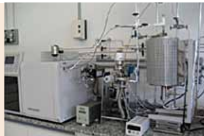
Evaluation unit of oxygen carrier in fixed-bed reactor coupled with gas chromatography and mass spectrometry.
